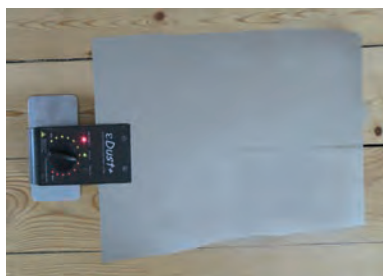
With fixed high voltage and ground connectors for lifting from floor (normal using).
